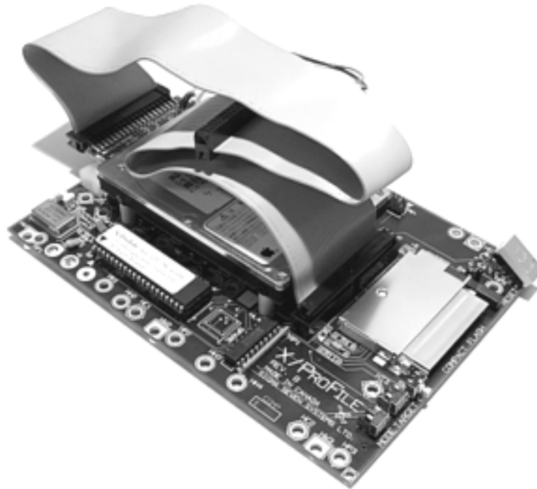
Figure 41. 2.5" drive, adapter and IDE cable mounted on X/ProFile
