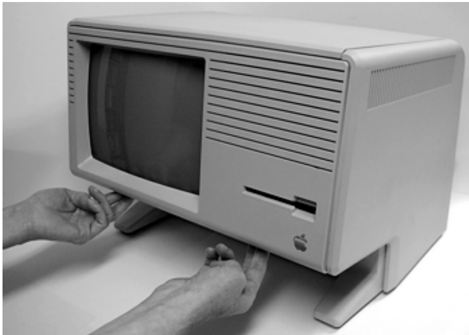
Figure 6. Releasing the X/Lisa front cover
