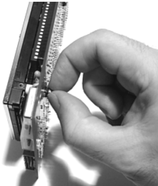
Figure 36. Attaching a 2.5" drive mounting screw
