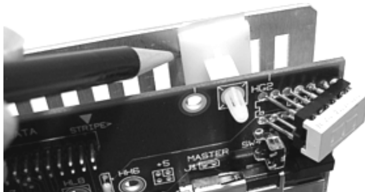
Figure 15. Marking the nylon mounting post locations
