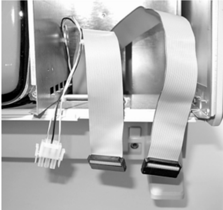
Figure 18. Lisa 2 drive cage cables
