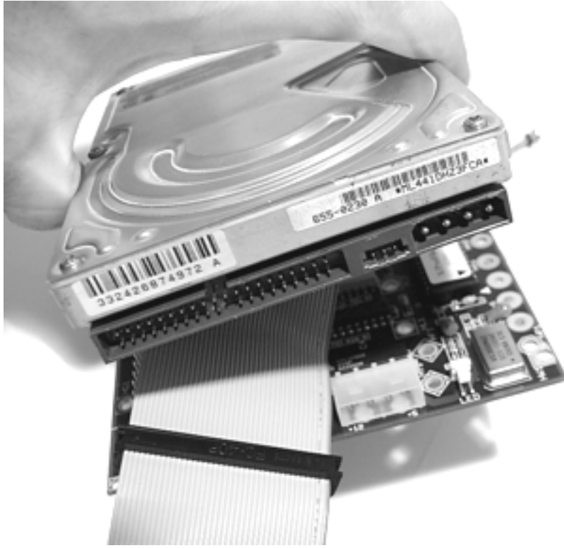
Figure 28. Orienting a 3.5" drive over the IDE cable
