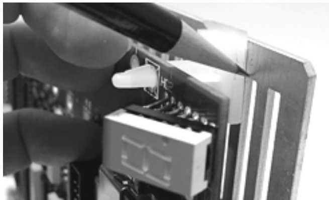
Figure 14. Marking the nylon mounting post locations
