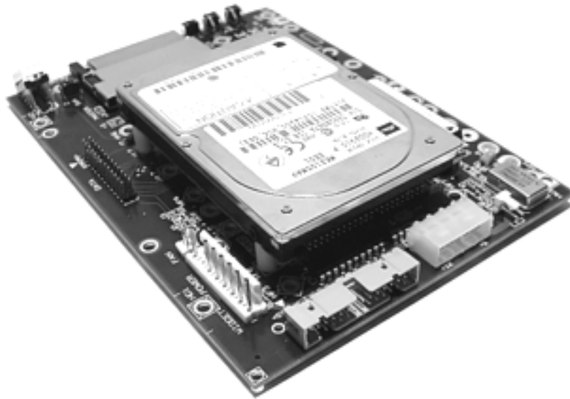
Figure 37. 2.5" drive mounted on X/ProFile
