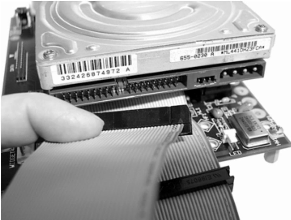
Figure 32. Attaching the IDE cable to the drive
