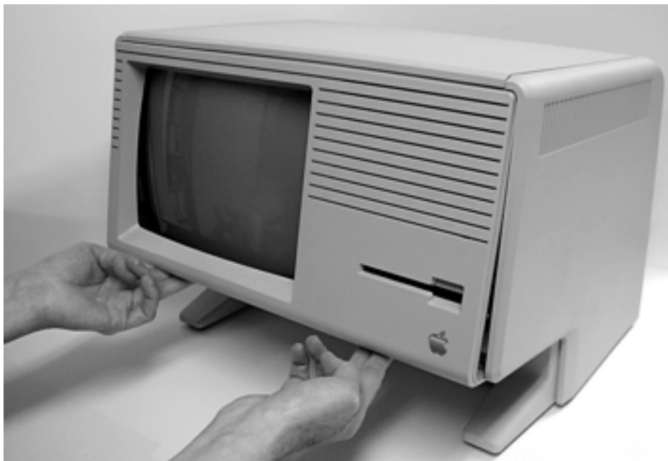
Figure 7. Removing the X/Lisa front cover
