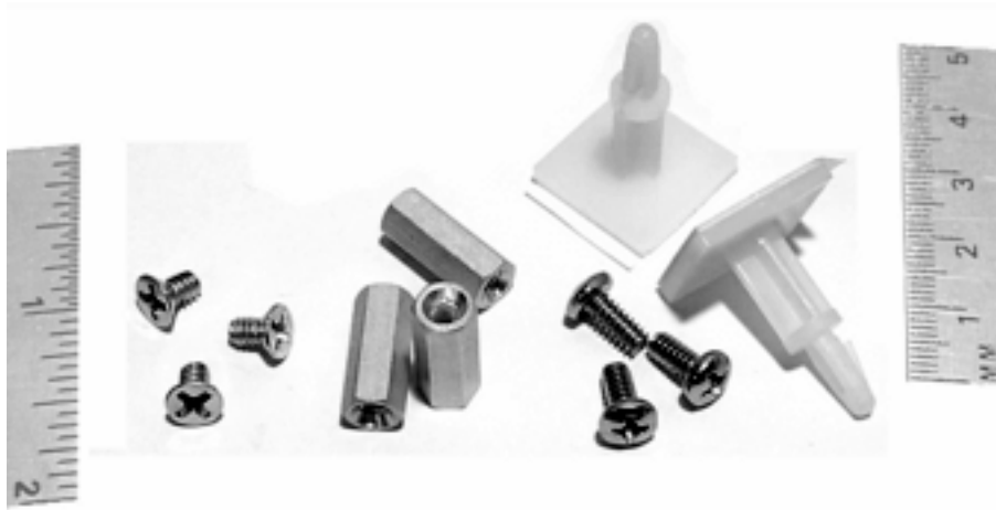
Figure 10. X/Lisa drive cage mounting hardware
