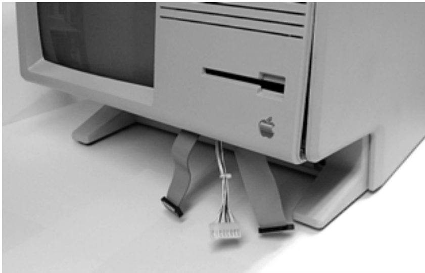
Figure 24. X/Lisa front cover ajar to permit start-up while cables are accessible
