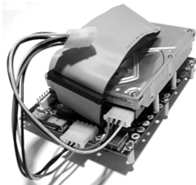
Figure 33. 3.5" drive and IDE cable mounted on X/ProFile
