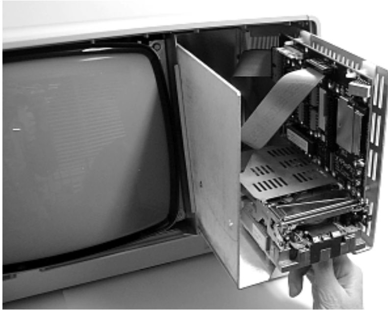
Figure 25. Replacing the X/Lisa drive cage
