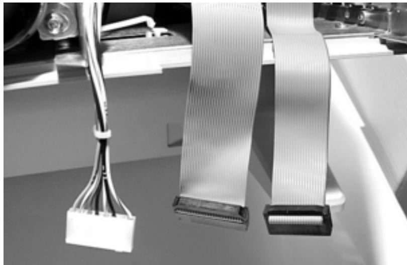
Figure 17. Lisa 2/10 and Macintosh XL drive cage cables
