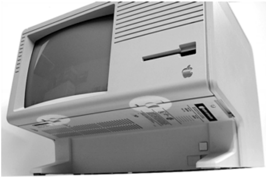
Figure 5. Locating the X/Lisa front cover latches
