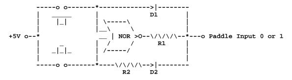
R1 = about 71K R2 = 150K D1 & D2 are switching diodes
